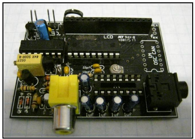
A COMPLETE ASSEMBLED FDIM2015 BUILDATHON FREQUENCY COUNTER BOARD FROM QRPme WAITING FOR CONFIGURATION MODS FOR THE DISPLAY.
